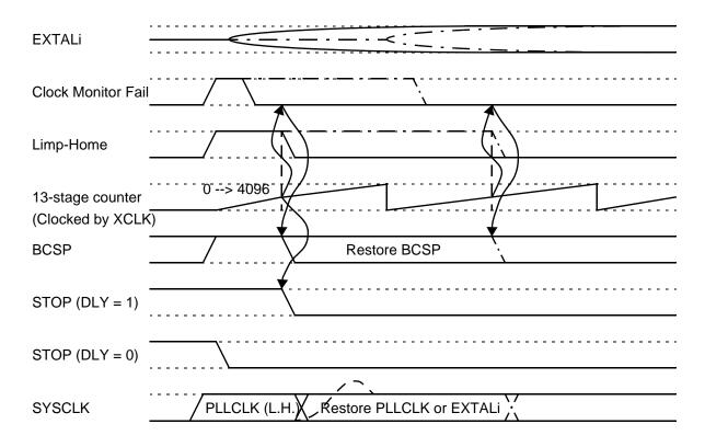
Figure 11-5. STOP Exit and Fast STOP Recovery
