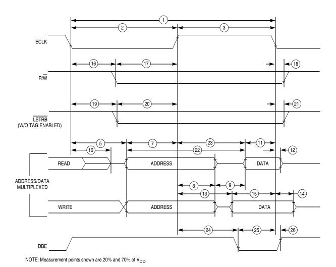
Figure 20-8. Multiplexed Expansion Bus Timing Diagram
