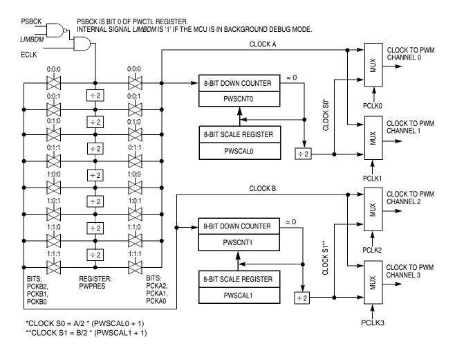
Figure 13-3. PWM Clock Sources
