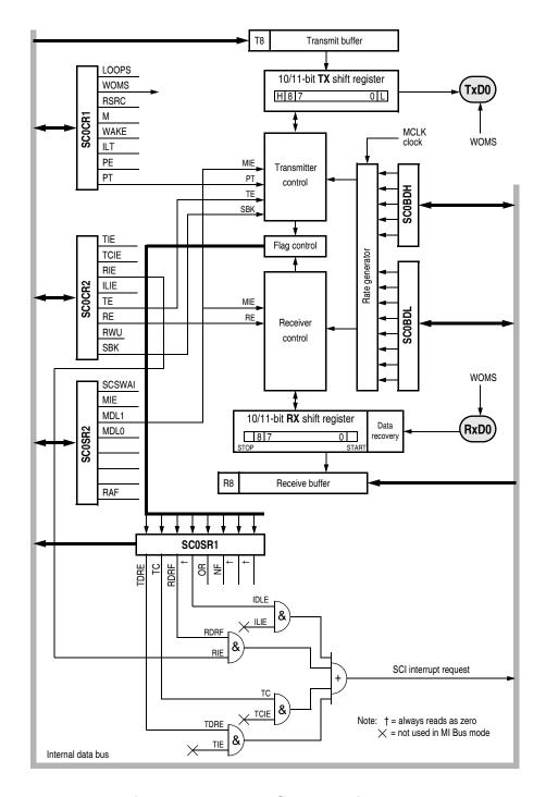
Figure 16-3. MI BUS Block Diagram
