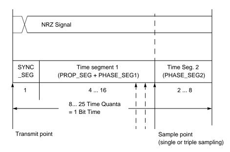
Figure 17-8. Segments within the Bit Time
