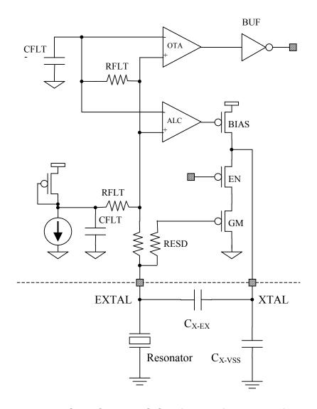
Figure 12-2. MC68HC912D60C Colpitts Oscillator Architecture
