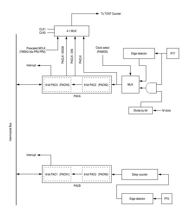
Figure 14-4. 16-Bit Pulse Accumulators Block Diagram
