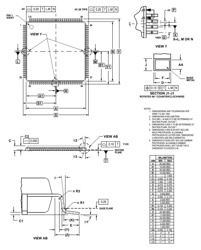
Figure 3-2. 112-pin TQFP Mechanical Dimensions (case no. 987)
