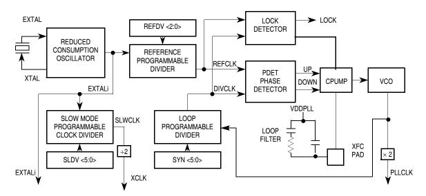
Figure 11-2. PLL Functional Diagram
