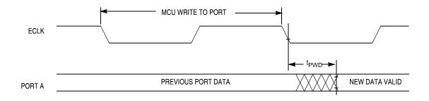
Figure 20-7. Port Write Timing Diagram
