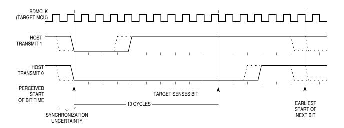
Figure 19-1. BDM Host to Target Serial Bit Timing
