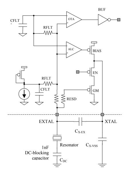
Figure 12-3. MC68HC912D60C Crystal with DC Blocking Capacitor
