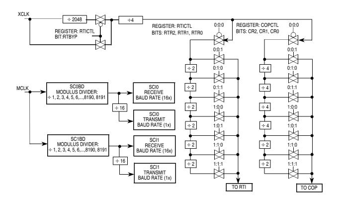
Figure 11-7. Clock Chain for SCI0, SCI1, RTI, COP
