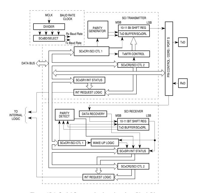
Figure 15-2. Serial Communications Interface Block Diagram
