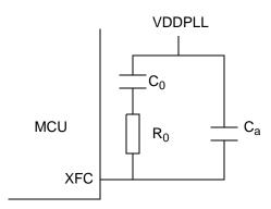
Figure 3-5. PLL Loop Filter Connections
