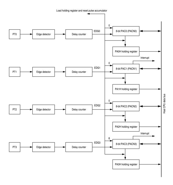
Figure 14-3. 8-Bit Pulse Accumulators Block Diagram
