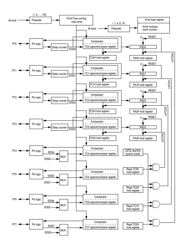
Figure 14-2. Timer Block Diagram in Queue Mode
