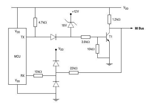
Figure 16-4. A typical MI Bus interface
