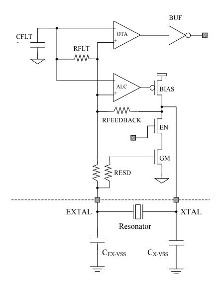
Figure 12-4. MC68HC912D60P Pierce Oscillator Architecture
