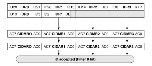
Figure 17-3. 32-bit Maskable Identifier Acceptance Filters
