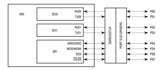
Figure 15-1. Multiple Serial Interface Block Diagram
