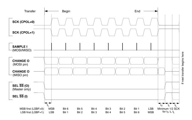
Figure 15-4. SPI Clock Format 0 (CPHA = 0)
