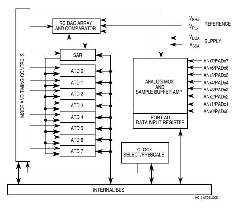
Figure 18-1. Analog-to-Digital Converter Block Diagram
