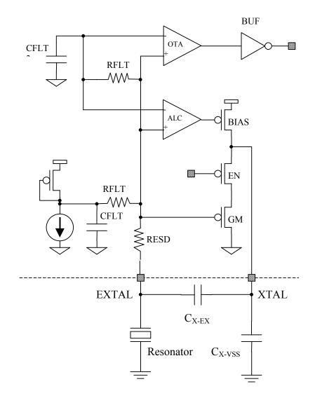
Figure 12-1. MC68HC912D60A Colpitts Oscillator Architecture
