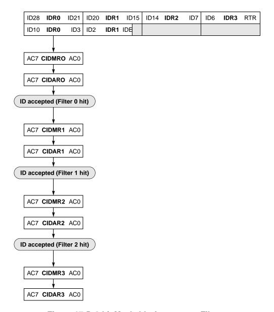
Figure 17-5. 8-bit Maskable Acceptance Filters
