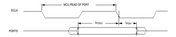
Figure 20-6. Port Read Timing Diagram
