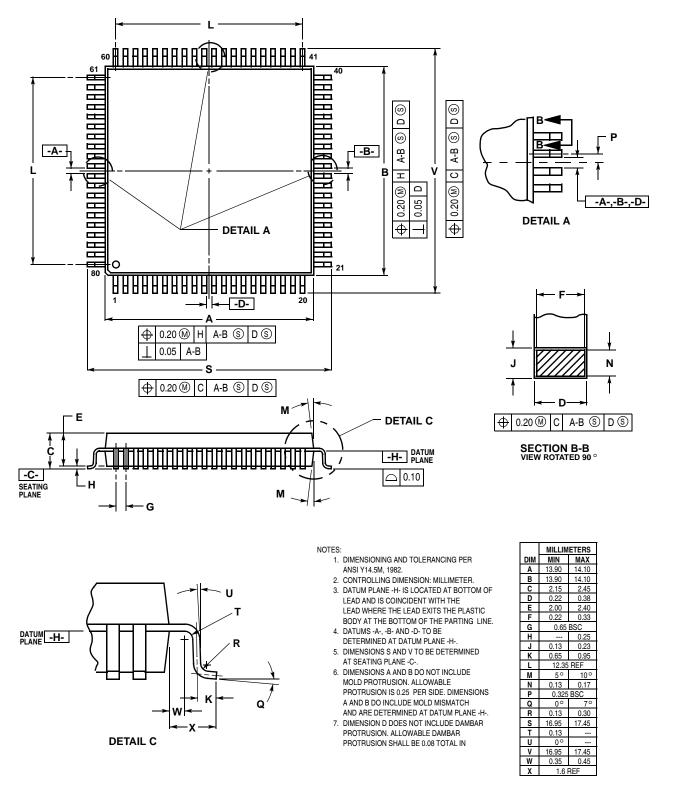
Figure 3-4. 80-pin QFP Mechanical Dimensions (case no. 841B)
