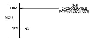
Figure 3-6. External Oscillator Connections
