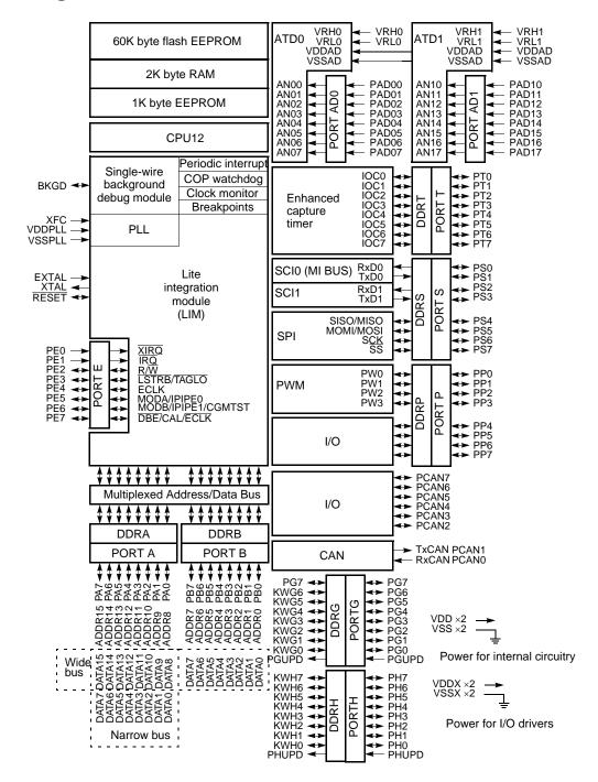
Figure 1-1. MC68HC912D60A 112-pin QFP Block Diagram
