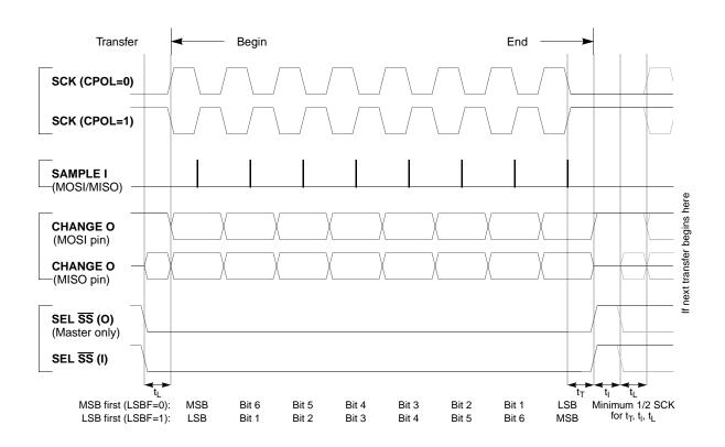
Figure 15-5. SPI Clock Format 1 (CPHA = 1)
