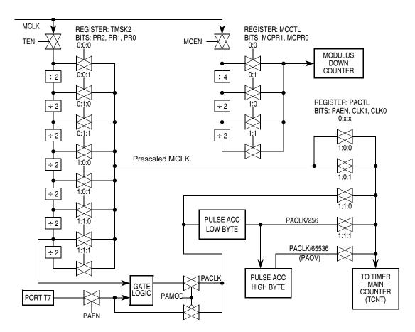
Figure 11-8. Clock Chain for ECT
