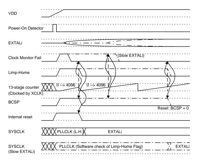
Figure 11-4. No Clock at Power-On Reset
