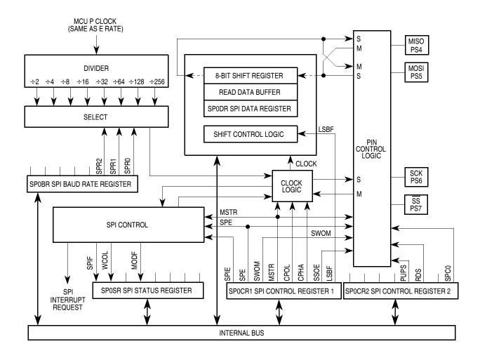
Figure 15-3. Serial Peripheral Interface Block Diagram
