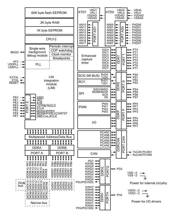
**Note:** Several I/O on ports G, H and CAN are unavailable externally on the 80-pin QFP package. These internal pins should either be defined as outputs or have their pull-ups/downs enabled.
