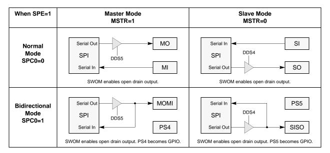
Figure 15-6. Normal Mode and Bidirectional Mode
