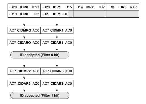
Figure 17-4. 16-bit Maskable Acceptance Filters
