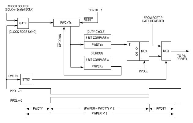
Figure 13-2. Block Diagram of PWM Center-Aligned Output Channel
