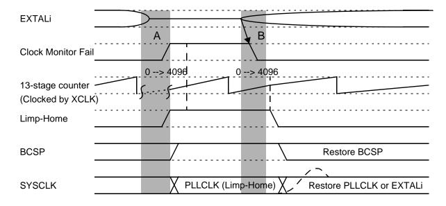
Figure 11-3. Clock Loss during Normal Operation
