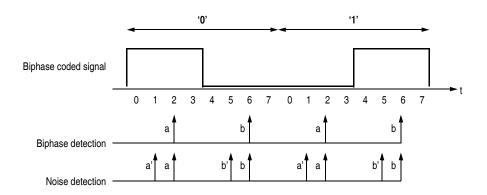
Figure 16-2. Biphase coding and error detection
