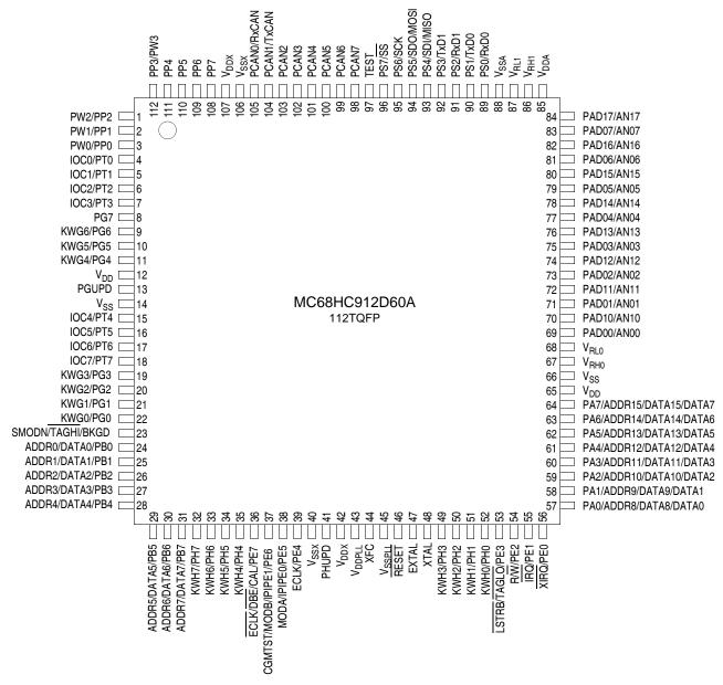
Note: TEST = This pin is used for factory test purposes. It is recommended that this pin is not connected in the application, but it may be bonded to 5.5 V max without issue.
